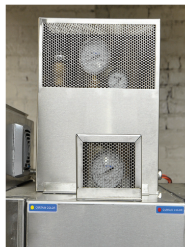
Shown above is the stainless steel perforated boxes used to protect the thermometers and gauges from damage.
