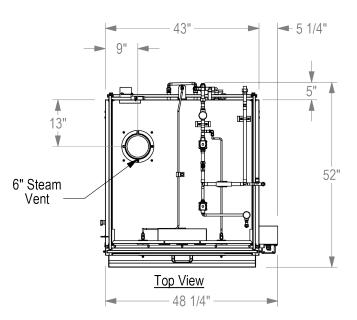
Note: Height with door open - 105 1/2" Door opening width - 39 1/4" Door opening height - 29 1/4"
